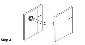
Install the other plate onto the wall, and slid two backings into the plate, make sure the 2 holes on the top.
