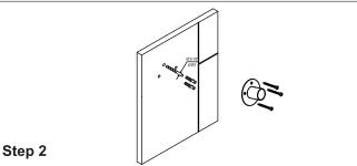
Predrill 3/16" holes on the wall to fit wall plugs, fix the plate onto the wall, make sure the post hole on the top.
