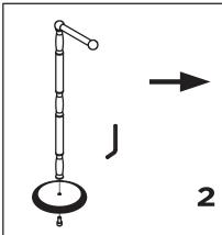
Align the tissue holder to the mouting holes on the bottom part, and use the Allen key to screw through from the back of the bottom and tighten it.
