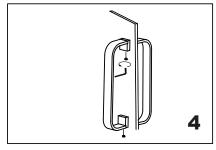
Fix the set screws on the end caps, tighten it to avoid loose from fixing brackets.
