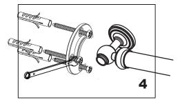
Driver bolt nut directly into holes
