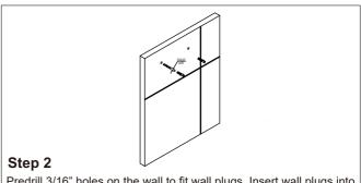
Predrill 3/16" holes on the wall to fit wall plugs. Insert wall plugs into the wall.
