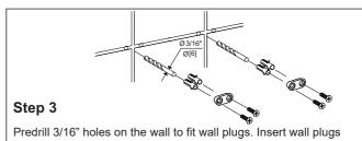
Predrill 3/16" holes on the wall to fit wall plugs. Insert wall plugs into the wall. Position backing plate flat side down over the plugs and install screws.
