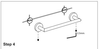
Slide the accessory onto the backing plates and tighten the set screws using Allen key provided.
