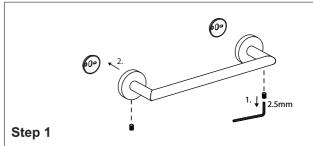
Loosen the set screw on the accessory and remove the backing plates. Position the accessory against the wall and mark outline with pencil.
