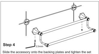
Slide the accessory onto the backing plates and tighten the s screws using Allen key provided.
