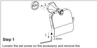
backing plate. Position the accessory against the wall and mark outline with pencil.
