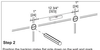
Position the backing plates flat side down on the wall and mark holes with pencil.
