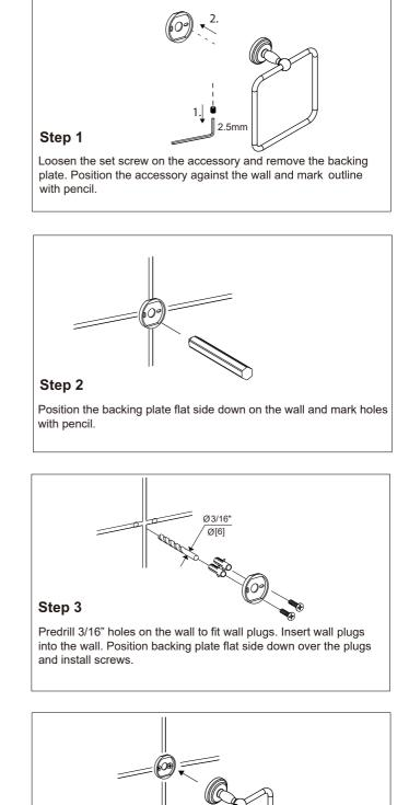
Slide the accessory onto the backing plate and tighten the set
