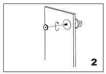
Screw in the fixing bracket into the hook bolt.
