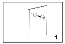
Install the hook (bolt) throught the glass hole, make sure the rubber gaskets are between knob&glass.
