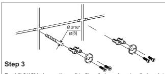
Predrill 3/16" holes on the wall to fit wall plugs. Insert wall plugs into the wall. Position backing plates flat side down over the plugs and install screws.
