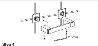
Slide the accessory onto the backing plate and tighten the set screw using Allen key provided.
