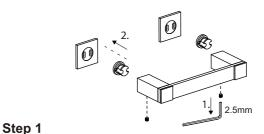
Loosen the set screw on the accessory and remove the backing plate. Position the accessory against the wall and mark outline
