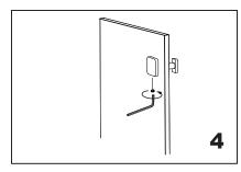
Fix the set screw on the end cap, tighten it to avoid loose from fixing brackets.
