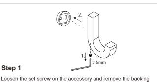
plate. Position the accessory against the wall and mark outline with pencil.
