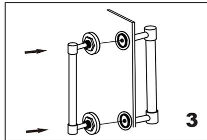
Add the handle B end caps on the fixing brackets, make sure the set screws holes in the bottom.
