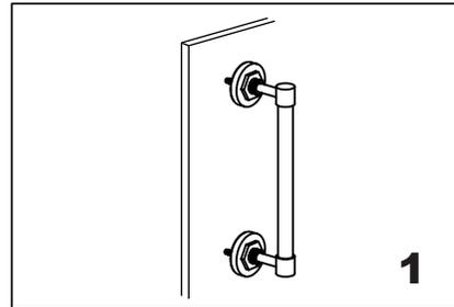
Install the handle A (bolt) through the glass holes, make sure the rubber gaskets are between handle & glass.
