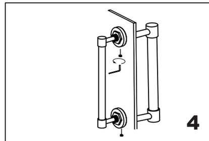
Fix the set screws on the end caps, tighten it to avoid loose from fixing brackets.
