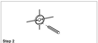
Position the backing plate flat side down on the wall and mark holes with pencil.
