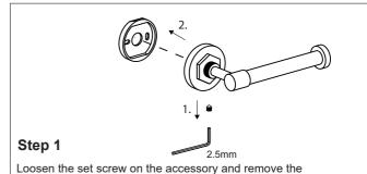
backing plate. Position the accessory against the wall and mark outline with pencil.
