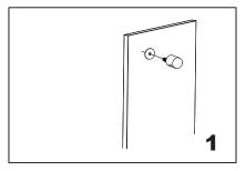
Install the knob-A (bolt) through the glass hole, make sure the rubber gaskets are between knob&glass.
