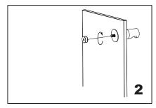
Screw in the fixing bracket into the hnob-A bolt.
