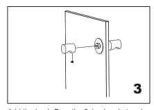
Add the knob-B on the fixing bracket,make sure the set screw hole in the bottom.
