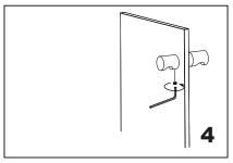
Fix the set screw on the knob-B, tighten it to avoid loose from fixing brackets.
