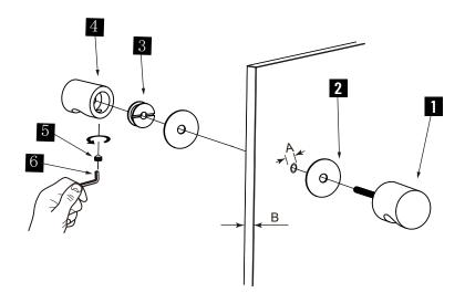
1.Knob-A x 1 2.Clear Gasket x 2 3.Fixing Bracket x 1 4.Knob-B x 1 5.Set Screw M5 x 1 6.Allen Key 2.5mm x 1
