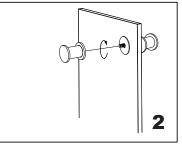
Screw in the knob-B into the bolt.
