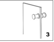
Tighten the knob-A & knob-B to avoid loosing.
