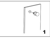
Install the knob-A (bolt) through the glass hole, make sure the rubber gaskets are between knob&glass.
