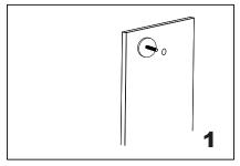
Install the end cap (bolt) through the glass hole, make sure the rubber gaskets are between end cap&glass.
