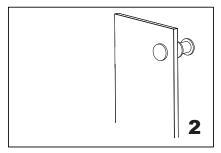
Screw in the knob into the hook bolt.
