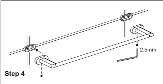
Slide the accessory onto the backing plate and tighten the set screw using Allen key provided.
