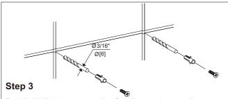
Predrill 3/16" holes on the wall to fit wall plugs. Insert wall plugs into the wall. Position backing plate flat side down over the plugs and install screws.
