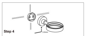
Slide the accessory onto the backing plate and tighten the set screw using Allen key provided.
