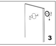
Add the end cap on the fixing bracket,make sure the set screw hole in the bottom.
