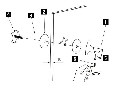
1.Knob x 1 2.Clear Gasket x 2 3.Fixing Bracket x 1 4.End Cap x 1 5.Set Screw M5 x 1 6.Allen Key 2.5mm x 1
