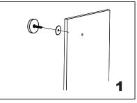
Install the knob (bolt) through the glass hole, make sure the rubber gaskets are between knob&glass.
