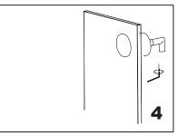
Fix the set screw on the end cap,tighten it to avoid loose from fixing brackets.
