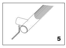
Tighten the post on the Mounting plate and fix with Allen Key
