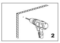
Drill 3/16" holes, make sure to keep drill level
