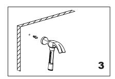
Insert plugs into drilled holes, using a hammer to tap the plugs in, be careful not to break tile
