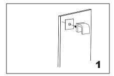
Install the knob (bolt) through the glass hole, make sure the rubber gaskets are between knob&glass.
