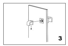
Add the end cap on the fixing bracket,make sure the set screw hole in the bottom.
